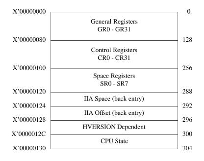
The "**Transfer Soft boot data**" option (ARG1=3) returns information about the processor state in the following format:
