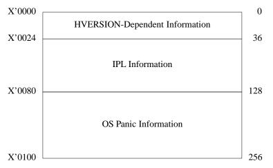
Providing Non-Volatile Memory is optional. If Non-Volatile Memory is provided, it must be at least 256 bytes in size and must be used for the architected purposes.
