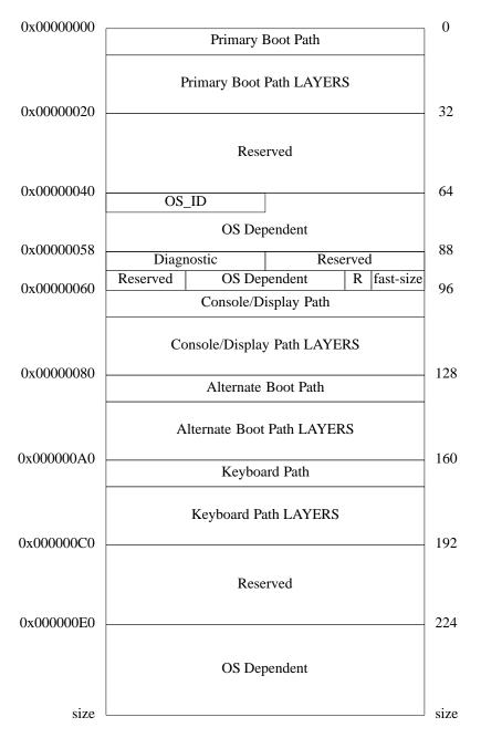
A minimum of 96 bytes of Stable Storage is required. Providing more than 96 bytes of Stable Storage is optional, but it must be used in the architected way if provided. Failure to provide the optional locations from 96 to 192 results in the loss of certain functionality during boot. (For example, ISL would not be able to set the console path.)
