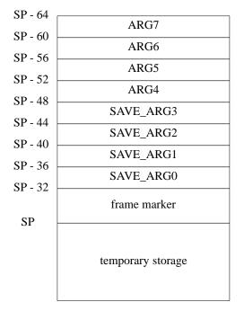
The values of SAVE\_ARG0 through SAVE\_ARG3 are defined by the caller at entry, and are unspecified at exit. They are used to save the first four arguments to the procedure, which are passed to the procedure in registers GR26 through GR23, respectively. Additional arguments are passed on the stack in successive locations (ARG8 at SP-68, ARG9 at SP-72, ARG10 at SP-76, etc.)
