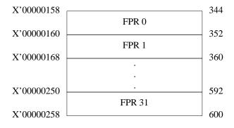
If software wants the address of these registers in memory to occur at doubleword-aligned boundaries, it must adjust the word-aligned *memaddr* parameter in the PDC\_PIM procedure to be doubleword aligned.
