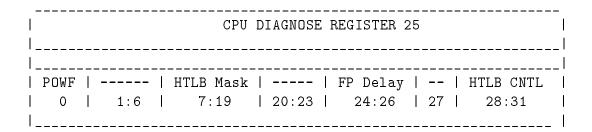
POWFAIL (r): Set to 0 by hardware when powerfail signal is true.
