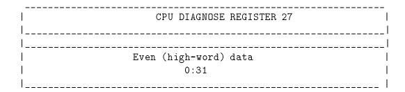
Diagnose Register 27, in the Level1 (on-chip) ICache is actually 2 different registers. Moves to this register set into one of the the ICache write latches to prepare for a Level1 ICache diagnose write. Moves from this register read one of the Level1 ICache read latches to complete a Level1 ICache diagnose read operation.
