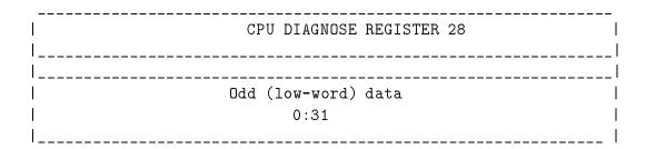
Diagnose Register 28, in the Level1 (on-chip) ICache is actually 2 different registers. Moves to this register set into one of the the ICache write latches to prepare for a Level1 ICache diagnose write. Moves from this register read one of the Level1 ICache read latches to complete a Level1 ICache diagnose read operation.
