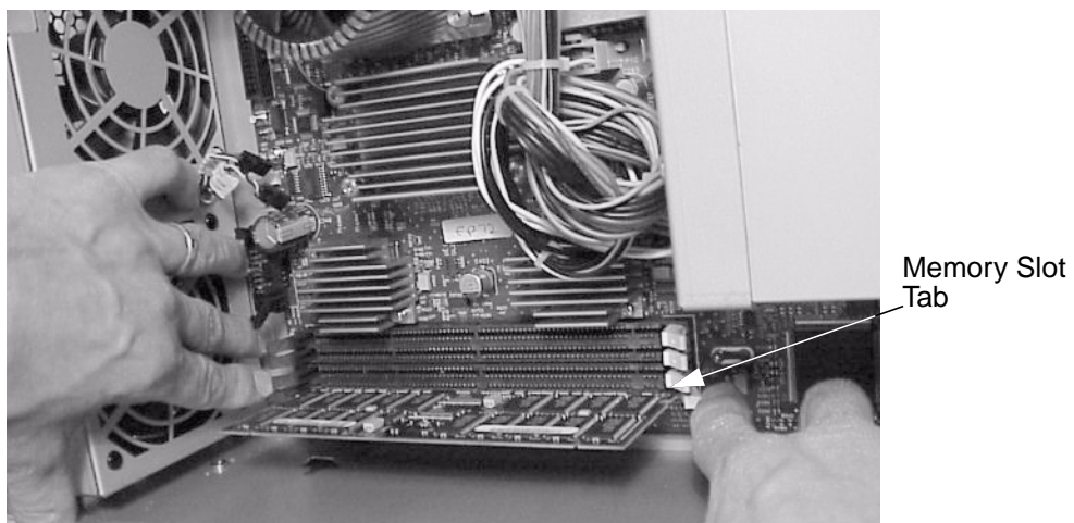
Figure 3-3. Pressing Down on the Memory Slot Tabs
