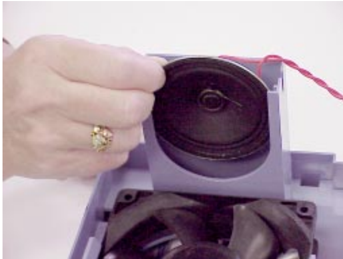
Figure 4-64. Removing the Speaker from the Mounting Bracket
