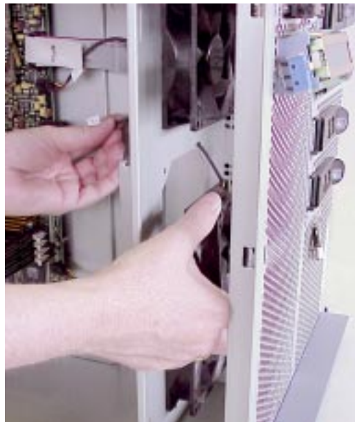
Figure 4-33. Threading the Fan Cable
