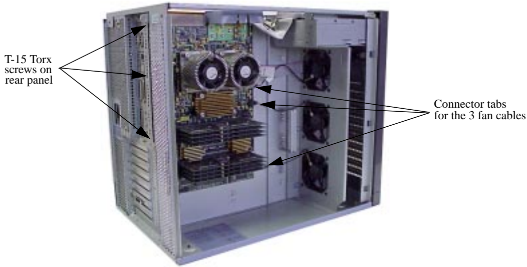
Figure 4-25. Fan Cable Connector Tabs and Rear Panel Screws
