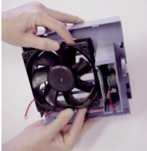
Figure 4-57. Removing the Fan from the Mounting Bracket
