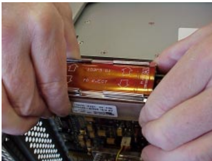
Figure 4-26. Connecting the Flex Cable
