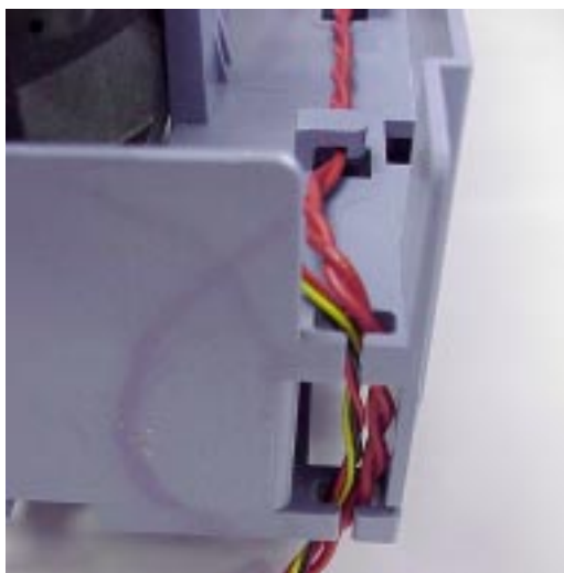
Figure 4-65. Threading the Fan Cable through the Plastic Slot
