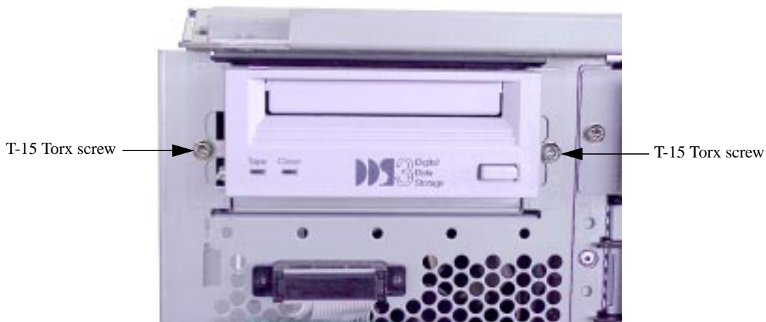
Figure 4-12. Front Panel Screws
