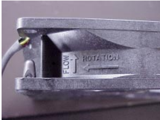
Figure 4-32. Fan Air Flow Arrow
