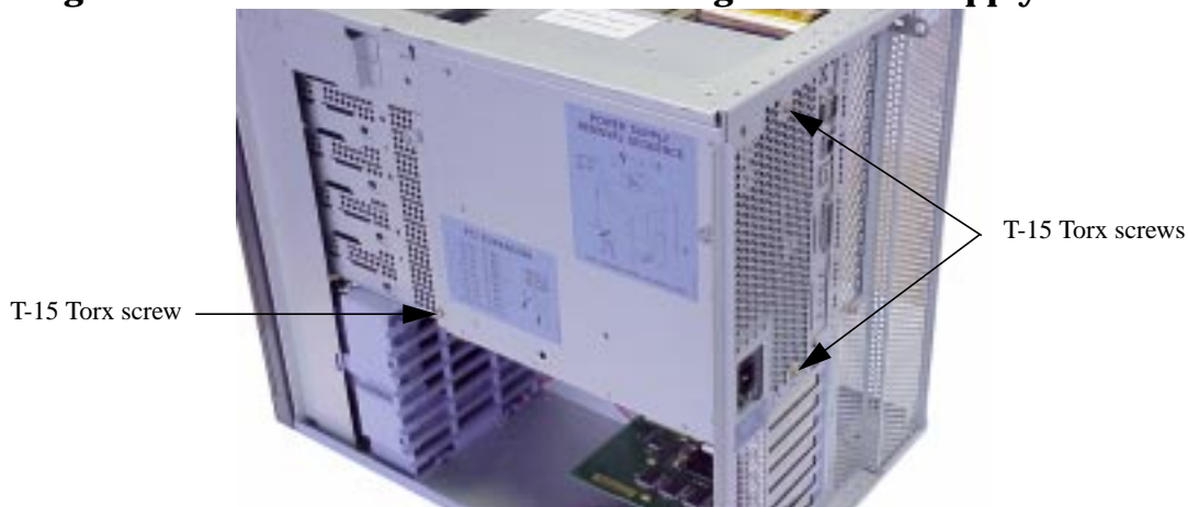
Figure 4-48. T-15 Torx Screws for Securing the Power Supply
