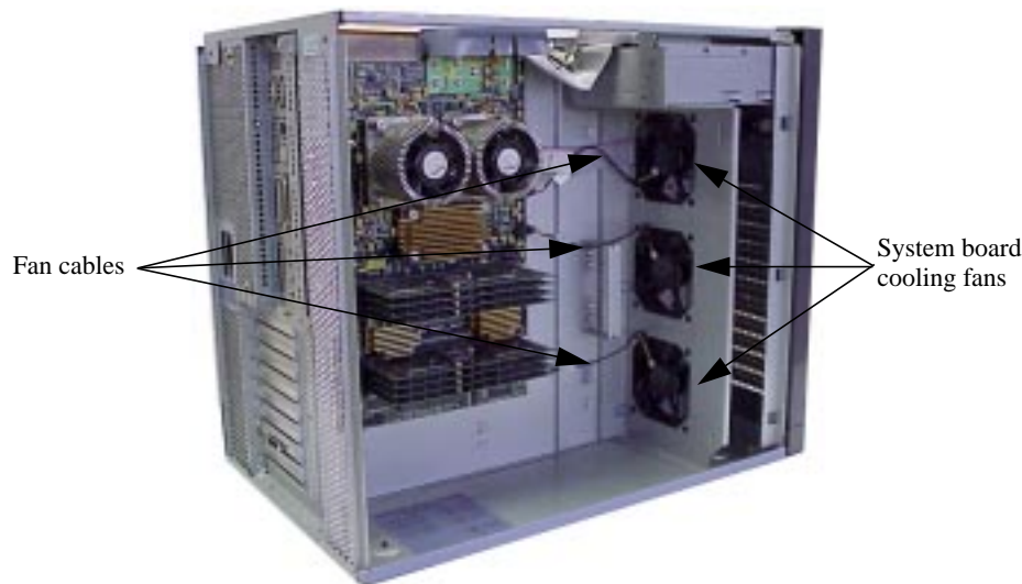
Figure 4-29. System Board Cooling Fans and Fan Cables
