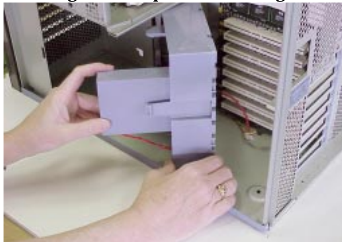
Figure 4-63. Removing the Fan/Speaker Mounting Bracket
