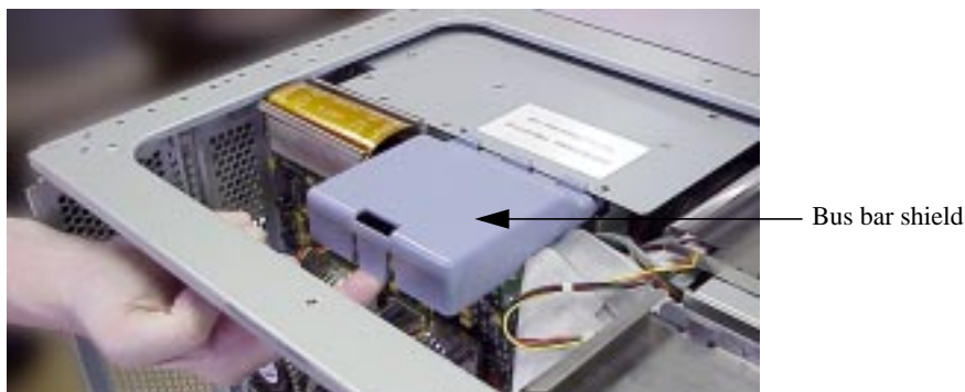
Figure 4-41. Removing the Bus Bar Shield
