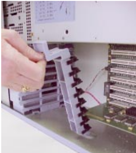
Figure 4-38. Removing the PCI Retainer Clip
