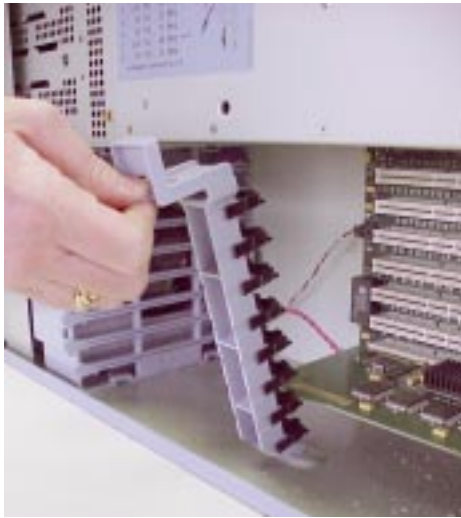
Figure 4-35. Removing the PCI Retainer Clip
