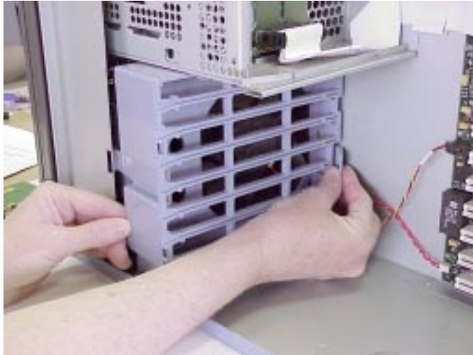
Figure 4-55. Loosening the Fan/Speaker Mounting Bracket
