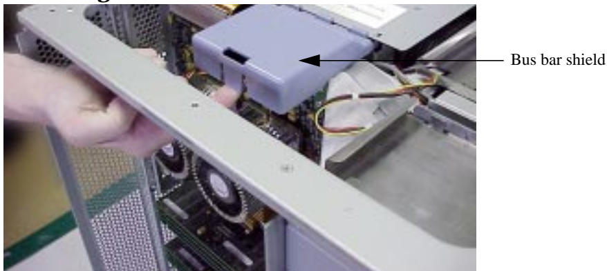
Figure 4-22. Removing the Bus Bar Shield
