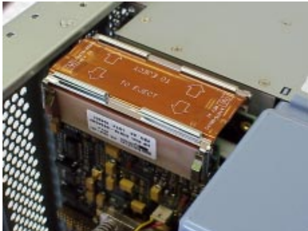
Figure 4-21. Arrows Indicate Where to Pull on the Ejector Handle
