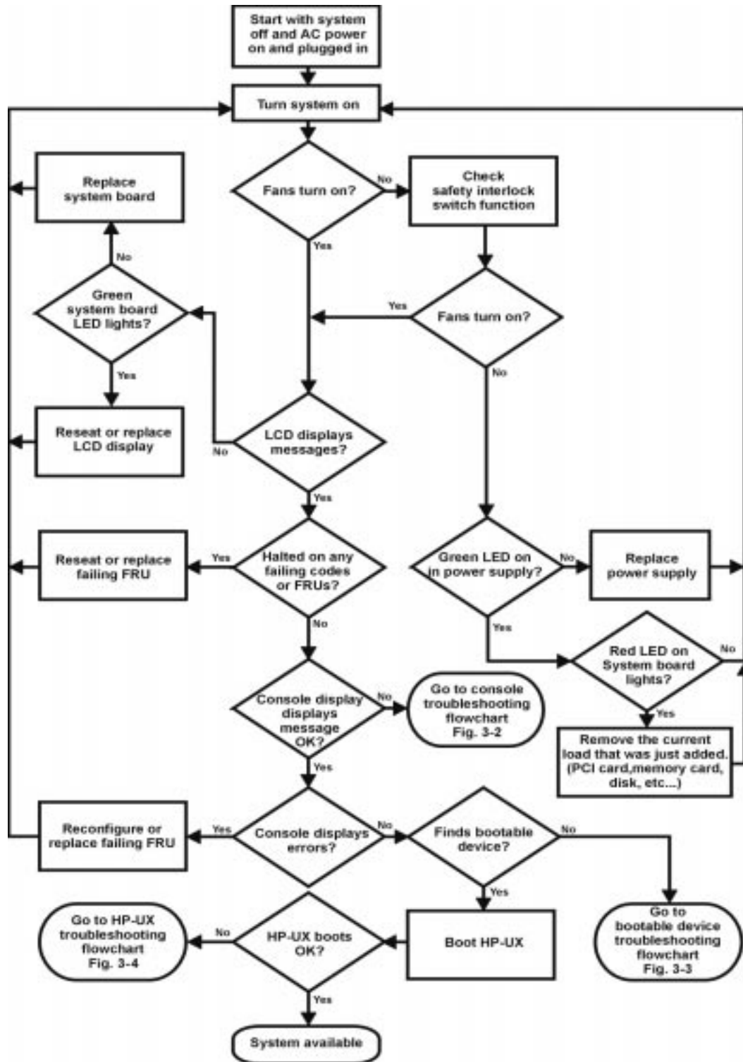
Figure 3-1. Power On LCD, Troubleshooting Flow
