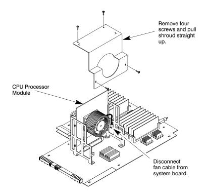
Figure B–28. Removing CPU Shroud and Disconnecting Fan Cable
