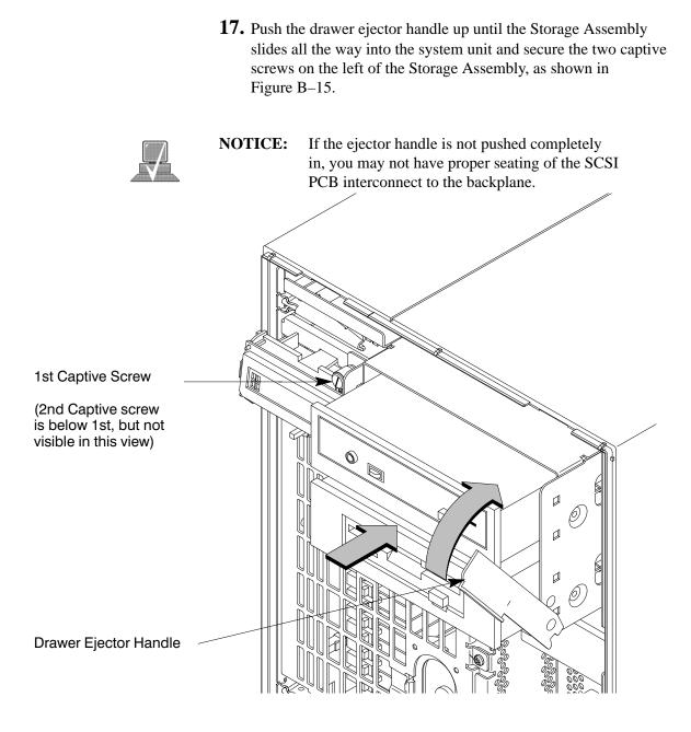
Figure B–15. Replacing the Storage Drawer Assembly
