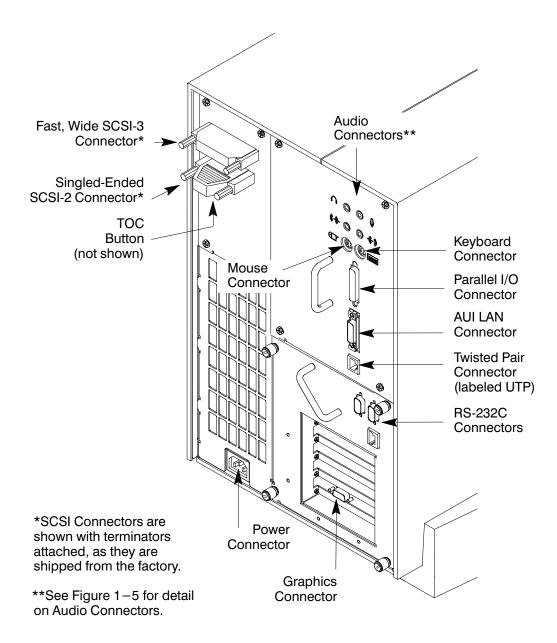
Figure 1-4. System Unit Rear Panel Connectors
