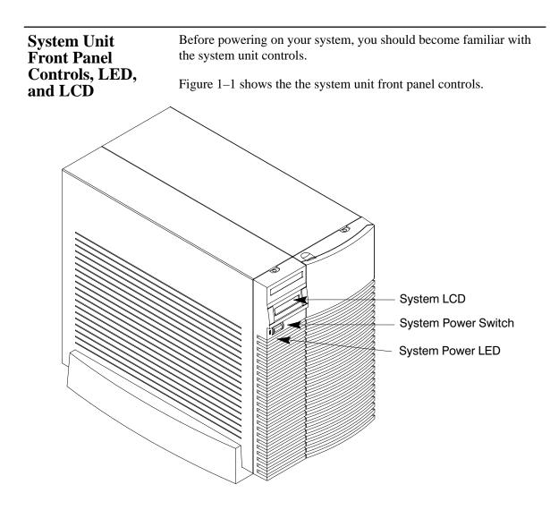
Figure 1–1. System Unit Front Panel Controls
