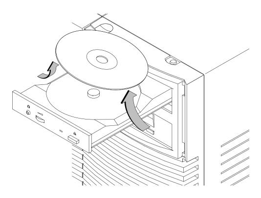
Figure 2–6. Removing the CD-ROM Disc From the Disc Tray
