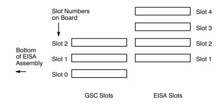
Figure B–32. EISA/GSC Slots from Inside the EISA Assembly
