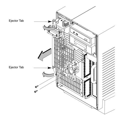
Figure B–20. Removing the CPU Assembly
