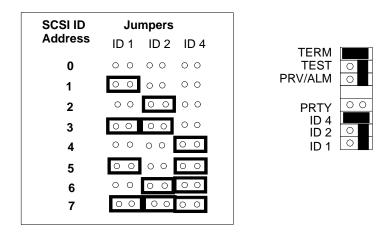
Figure B–7. CD-ROM Drive SCSI Address/Jumper Settings
