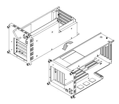
Figure B–39. Rotating the EISA Assembly Back
