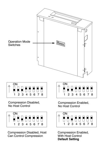
Figure B–10. Switch Settings for Data Compression Operation Mode
