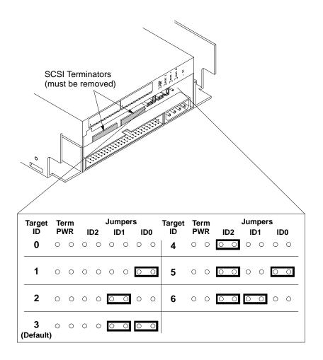
Figure B-8. DDS-DC Tape Drive SCSI Address/Jumper Settings
