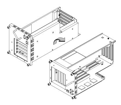
Figure B–34. Rotating the EISA Assembly for Installation
