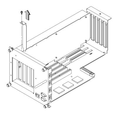
Figure B–36. Removing the EISA Slot Cover
