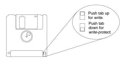
Figure 4–1. Setting the Write-Protect Tab on a Floppy Diskette
