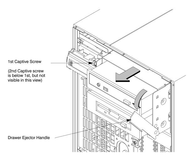
Figure B–18. Removing Storage Drawer from System Unit
