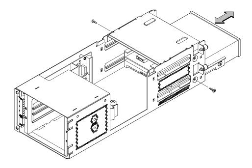
Figure B-6. Removing Drive Screws
