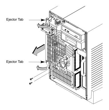
Figure B–26. Removing the CPU Assembly
