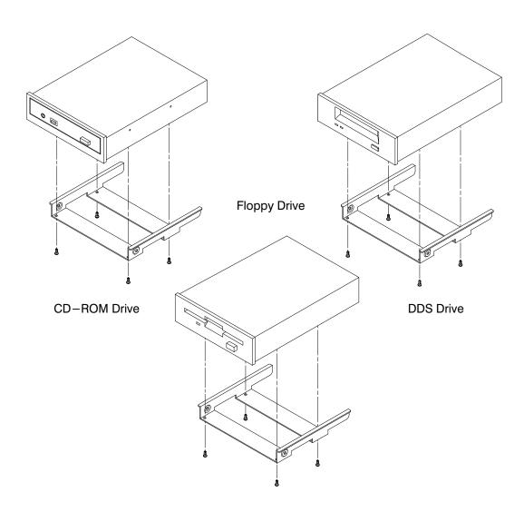
Figure B–13. Attaching Removable Drive Mounting Bracket and Drive Orientation
