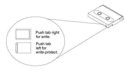
Figure 3–2. Setting the Write-Protect Tab on a DDS Tape
