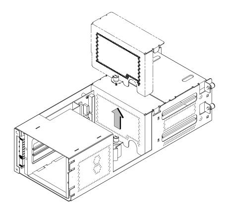
Figure B–5. Removing FAN/EMI Plate
