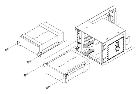
Figure B–19. Placing Hard Drives in Storage Drawer
