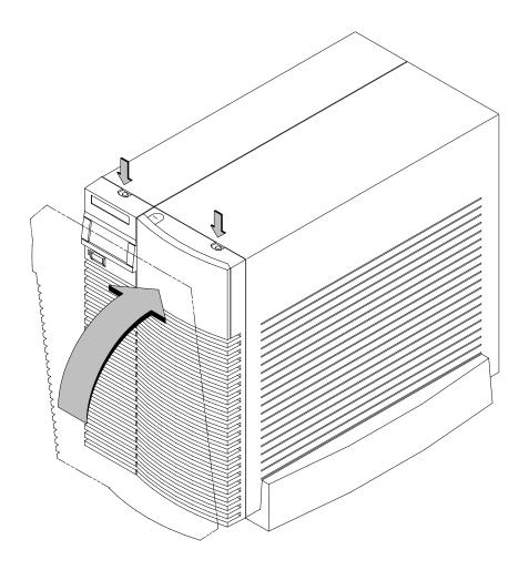
Figure B–2. Replacing the Front Panel
