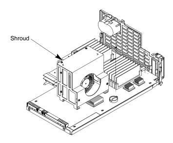
Figure B-27. CPU Shroud Location
