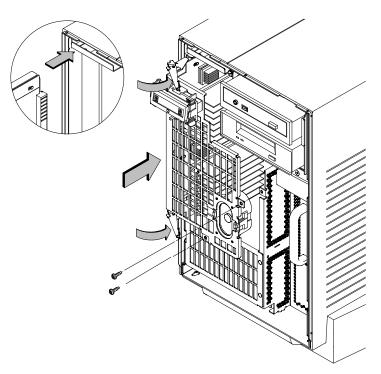
Figure B–30. Replacing the CPU Assembly
