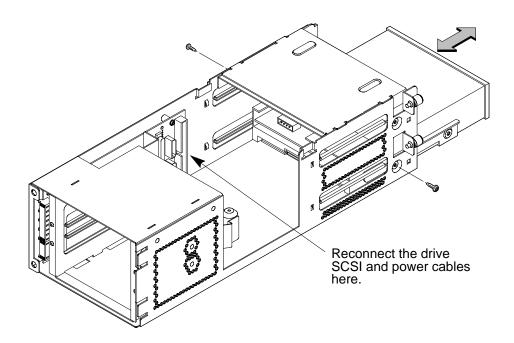
Figure B-14. Replacing Drive Screws
