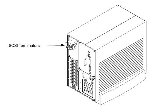
Figure C–1. Rear Panel SCSI Connectors with Terminators Attached
