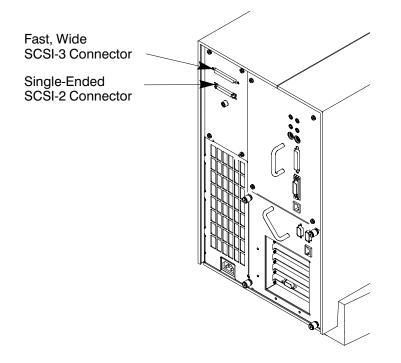
Figure C-2. Rear Panel SCSI Connectors without Terminators
