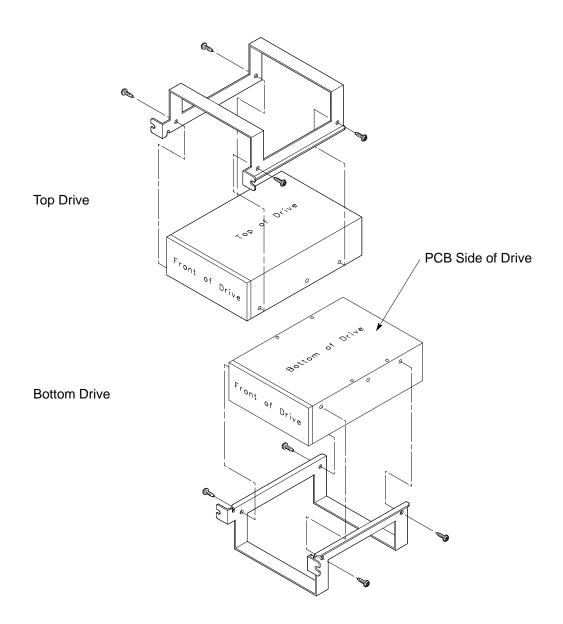
Figure B–17. Replacing Hard Drive Mounting Bracket and Drive Orientation
