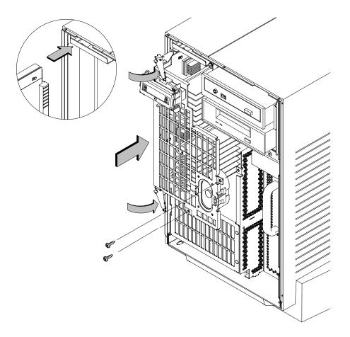
Figure B–25. Replacing the CPU Assembly
