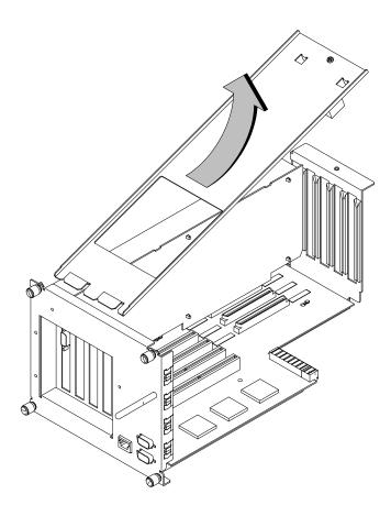
Figure B–35. Removing the EISA Assembly Cover
