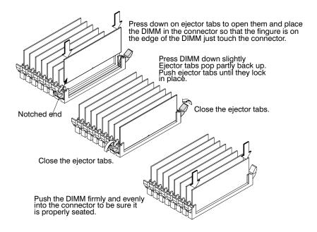
Figure B-24. Installing Memory Cards
