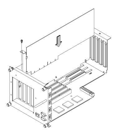
*Figure B–37. Installing an EISA or Graphics Board in the EISA Assembly*
