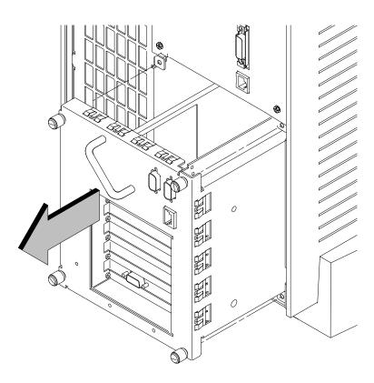
Figure B–33. Removing the EISA Assembly
