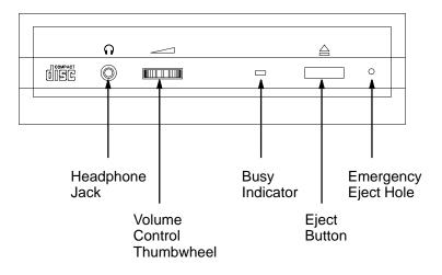
Figure 2–1. CD-ROM Drive Controls and Features
