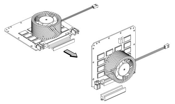
Figure B–29. Removing CPU Dust Cover
