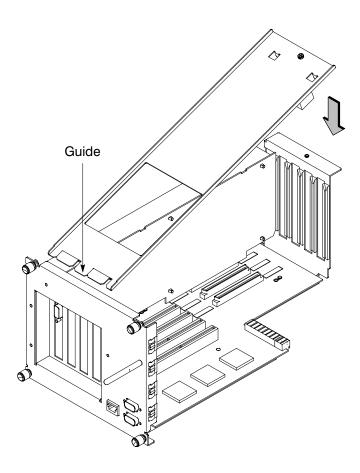
Figure B–38. Replacing EISA Assembly Cover
