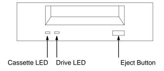
Figure 3–1. DDS Drive Controls and Indicators
