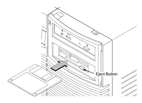
Figure 4–2. Inserting and Removing a Floppy Diskette
