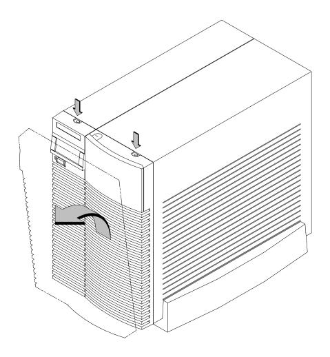
Figure B–1. Removing the Front Panel
