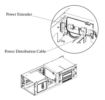
Figure B–4. Removing EMI Plate
