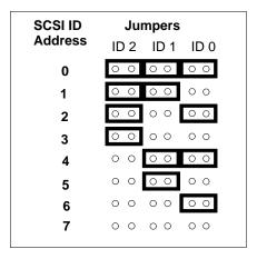
Figure B–11. Floppy Drive SCSI Address/Jumper Settings
