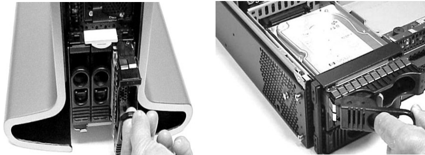
Removing the Hard Disk Drive from the System
