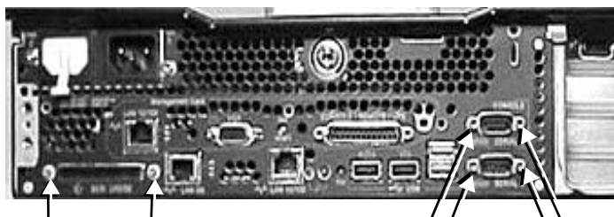
Six System Board Mounting Screws
