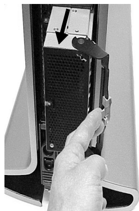
Removing the Power Supply from the System
