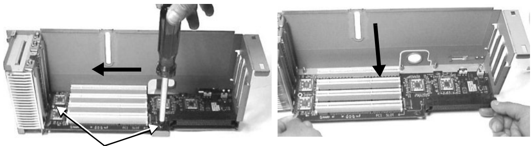
Removing the PCI/AGP backplane (rx2600 shown)
