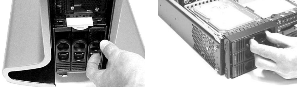
Squeezing Inward on the Hard Drive Release Clip
